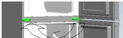
8. Set the bottom door right position,fix the mid-hinge.
